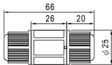
CJ04-1 suitable for 14AWG~16AWG
