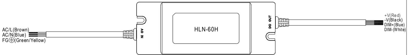
※ Built-in 3 in 1 dimming function, IP64 rated. Output constant current level can be adjusted through output cable by connecting a resistance or 1 ~ 10Vdc or 10V PWM signal between DIM+ and DIM-.
