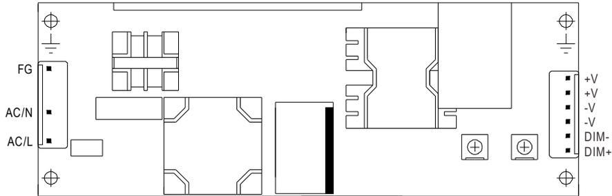
※ Output constant current level can be adjusted through output connector by 1~10VDC, PWM signal, or connecting a resistance between DIM+ and DIM-.
