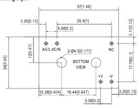
Case No.IRM03 Unit:mm[inch] Tolerance:±0.5[±0.02] unless otherwise specified
