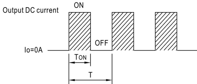
$$\text{Duty cycle(\%)} = \frac{T_{\text{ON}}}{T} \times 100\%$$
