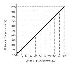
$\bigcirc$  Applying additive 10V PWM signal (frequency range 100Hz ~ 3KHz):
