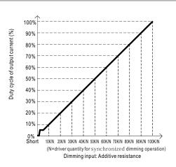
Note: 1. Min. duty cycle of output current is about 6% and the output current is not defined when 0% Iout<6%. 2. The duty cycle of output current could drop down to 0% when dimming input is about 0% or 0% or 0% or 0% or 0% duty cycle.
